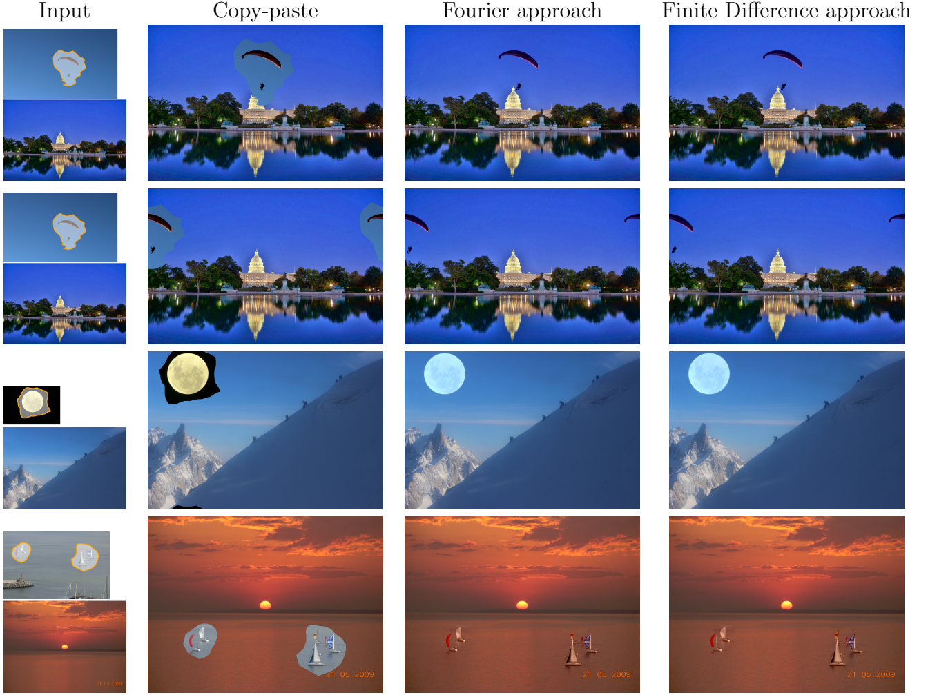
Figure 18: Examples of seamless cloning with the described numerical methods.
