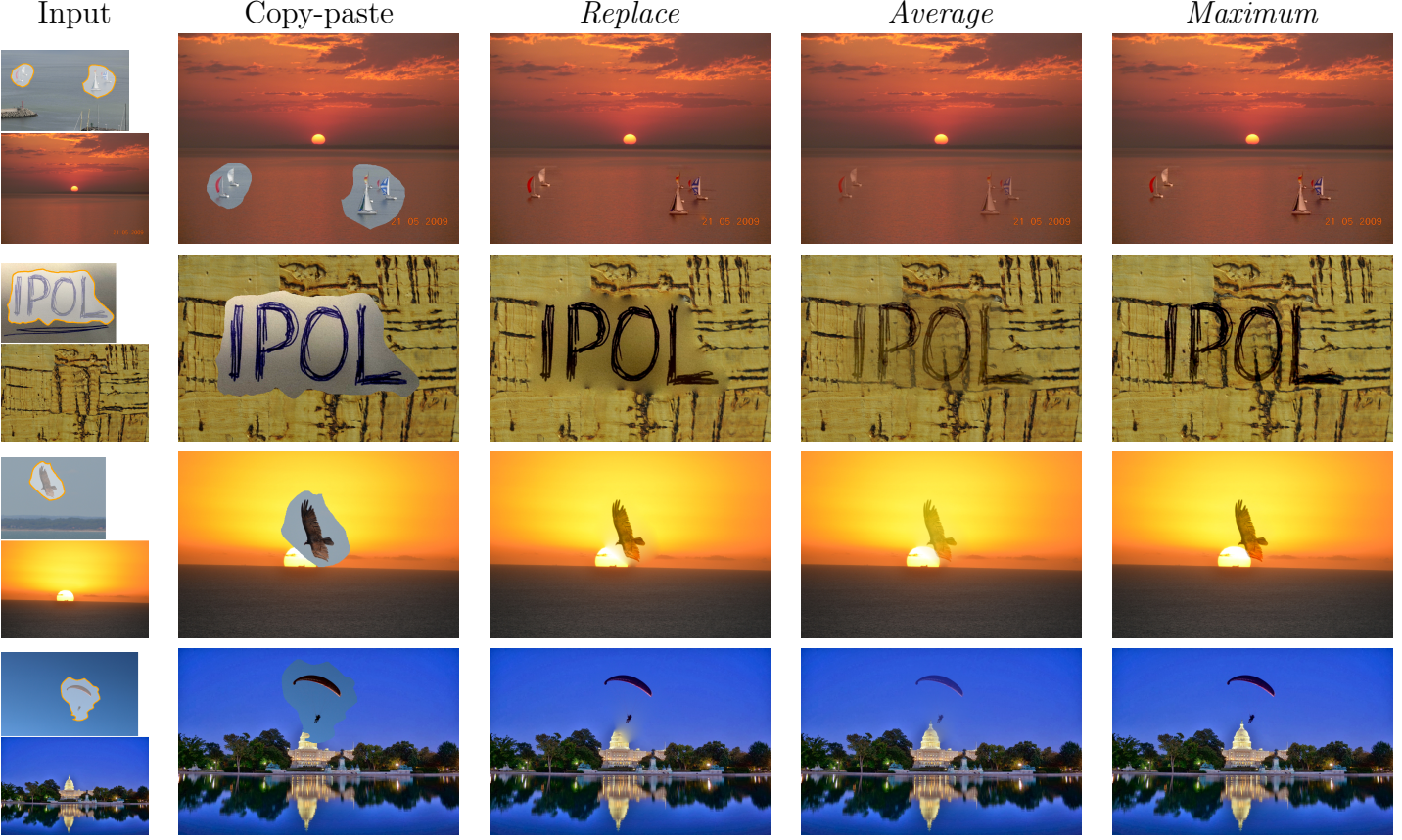
Figure 12: The first column shows the input images and the selected domain, the second column shows the result of copy-pasting the selected region over the destination image. The third column shows the result of replacing the gradients ( \mathbf{v} = \nabla I_1 ), the fourth column the result of averaging source and destination gradients i.e. \mathbf{v} = 1/2(\nabla I_1 + \nabla I_2) , and finally the last column corresponds to keeping the maximum gradient between the source and destination images. These results were obtained using the finite difference numerical method .
